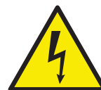
Caution Risk of Electric Shock
