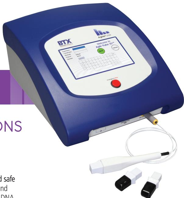
**Simple User Interface** – Touch screen user interface, USB key data storage, and Windows® Mobile 6.0 operating system. The system automatically stores a digitized record of all pulse parameters for quality control. EN 60601-1, EN 60601-1-1 EN 60601-1-2, UL60601-1 and CSA 601.1 compliant.
